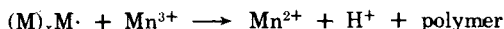
Scheme I: glycol cleavage mechanism with Mn 3+ ions leading to initiation of graft copolymerization
